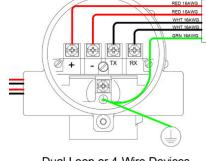
Dual Loop or 4-Wire Devices ZeroDT 24-2 & ZeroDT 12-2 2 Red Wire ( Voltage + or - ) 2 White Wire ( Voltage + or - ) 1 Green Wire (GND)
