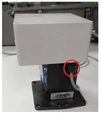
The other end of the interfacing cable (40-6189) runs to the Pulsar Output gland.
