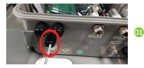
Insert the interfacing cable (40-6189) from the Pulsar through the Pulse Input Gland on MIWI350 device.
