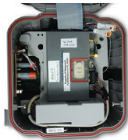
When used in the EC350, the Cloud Link 4G Modem requires no external antenna
