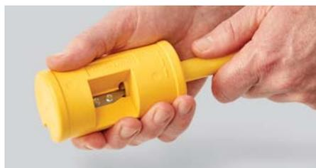
4. Insert tube and rotate in chamfer tool until tube bottoms out.
