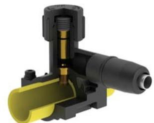
4. Cap is threaded onto tower. PermaLock tapping tees provide a .80" port for high gas flow (.55" in 1-1/4" mains).
