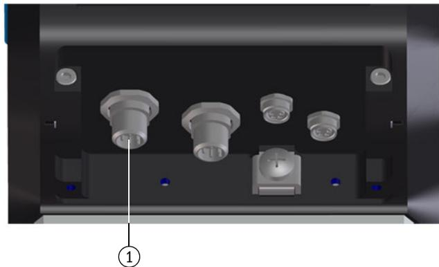
1 External power supply and signal output
