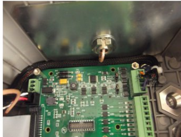
Route cables in the orientations as shown, before re-assembling HF cover
