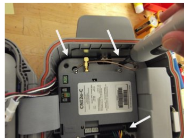
Tighten screws to 8-10 in-lbs
