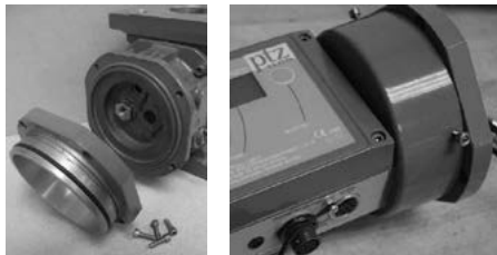
Figure 2 – IMC/W2 Meter Mounting Guide - Series B
