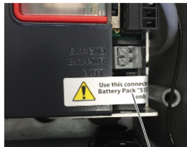
Cloud Link 4G Modem battery connector
