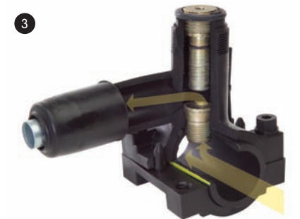
Cutter is reversed until flush with the top of tower. Locking sleeve remains permanently threaded into the gas main.
