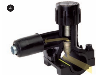
Cap is threaded onto tower. PermaLock tapping tees provide a .80" port for high gas flow (.55" in 1-1/4" mains).
