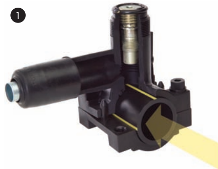
PermaLock full-encirclement tee is bolted onto the main.
